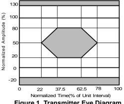
Figure 1. Transmitter Eye Diagram
