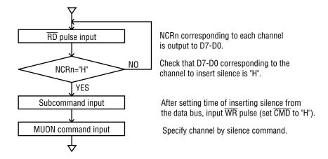
Figure 9-3 MUON Command Input Flow
