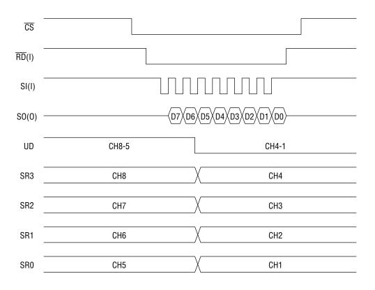
Figure 8-2 Read timing in serial input interface
