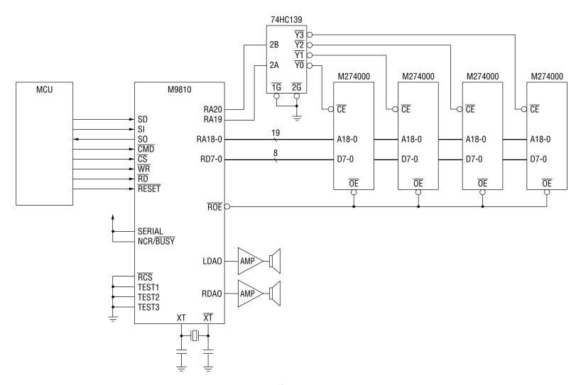
Application circuit example when four 4Mbit EPROMs are connected (serial interface)
