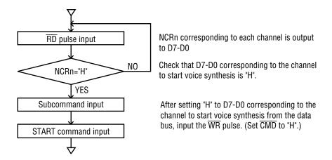
Figure 9-1 START Command Input Flow
