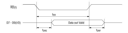
Figure 7-2 Parallel input read cycle timing
