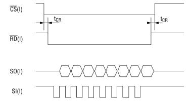
Figure 7-4 Serial input read cycle timing
