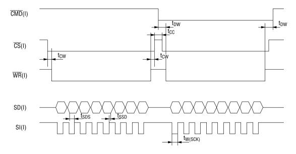
Figure 7-3 Serial input write cycle timing
