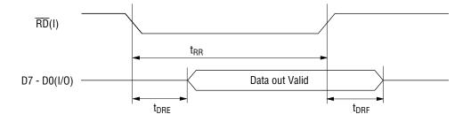
Figure 8-1 Read timing in parallel input interface
