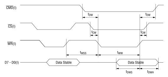
Figure 7-1 Parallel input write cycle timing
