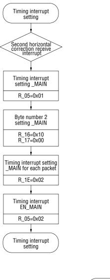
(2) Checking the byte number and the packet number of Figure 5.3
