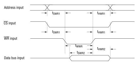
Figure 4.1 Write Timing
