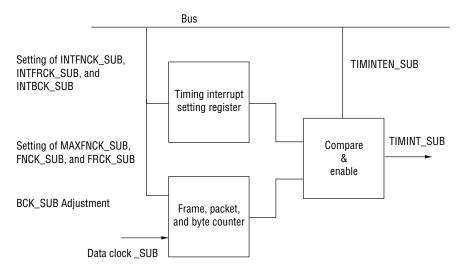
Figure 5.4.2 TIMINT\_SUB block diagram
