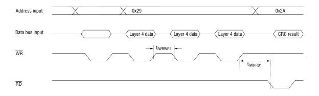
Figure 4.3 Layer 4 CRC mode and Layer 4 VICS mode Timing
