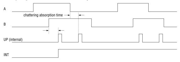
Fig.2 The Input and Output Timing in Case of Clockwise.
