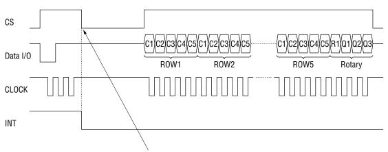
When CS goes L, the up/down counter is reset and the INT goes "L".
