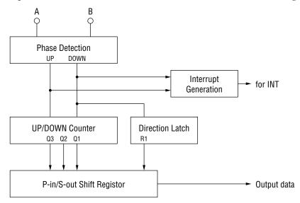
Fig.1 The Rotary Encoder Switch Circuit
