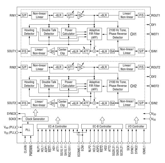
The above diagram shows internal connections for 2-channel parallel mode. The internal connections for 2-channel serial I/O mode and 1-channel cross-connected mode are shown below.
