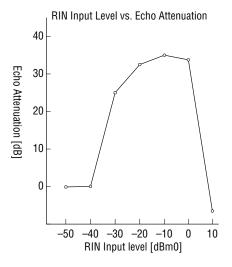
Measuring Conditions: RIN input = white noise Echo delay time = 50 ms E.R.L. = 6 [dB] ATT, GC, NLP, LR all off
