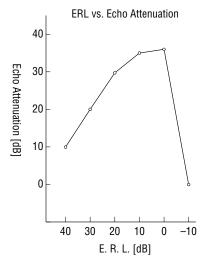
Measuring Conditions: RIN input level = -10 dBm0 white noise Echo delay time = 50 ms ATT, GC, NLP, LR all off
