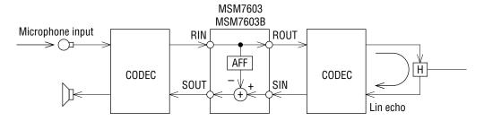
Example 3: Canceling of both acoustic and line echo (to handle both acoustic echo from line input and line echo from microphone input)
