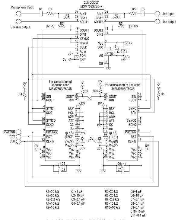
Use the MSM7704-01GS-VK as a PCM CODEC when  $V_{DD}$  3 V is used. The MSM7533 is pin compatible with the MSM7704.
