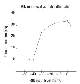
Measurement Conditions : RIN input = -10 dBm0 5 kHz band white noise Echo delay time  $T_D$  = 50 ms ATT, GC, NLP = OFF Power supply voltage 5 V
