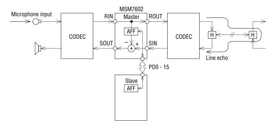
Example 4: Canceling of both acoustic echo and line echo (to handle both acoustic echo from line input and line echo from microphone input)
