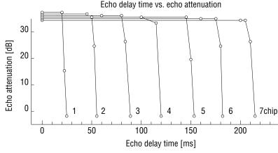
Measurement Conditions RIN input = -10 dBm5 kHz band white noise (0 dBm = 2.2 dBm0)
