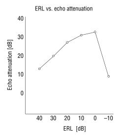
Measurement Conditions RIN input = -10 dBm 5 kHz band white noise (0 dBm = 2.2 dBm0)Echo delay time  $T_D = 20 \text{ ms}$ ATT, GC, NLP = OFF Power supply voltage 5 V
