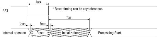
Note:  $\overline{\text{INT}}$  is invalid in the diagonally shaded interval.
