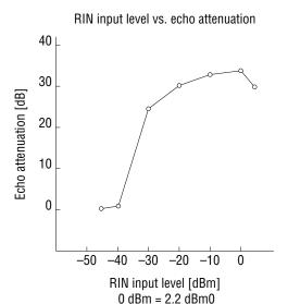
Measurement Conditions RIN input: 5 kHz band white noise Echo delay time  $T_D = 20 \text{ ms}$ ERL = 6 dBATT, GC, NLP = OFF Power supply voltage 5 V
