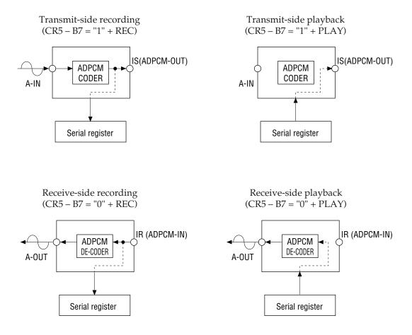
Figure 20 Signal Flow in Transmit/Receive Side Recording/Playback
