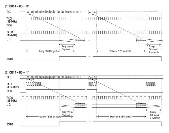
Figure 3 Transmit Timing Diagram
