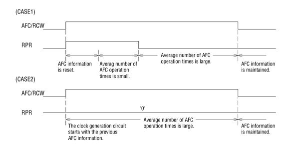
Figure 5 AFC Control Timing Diagram
