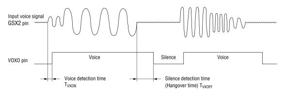
(a) Transmission Side VOX Function Timing Diagram
