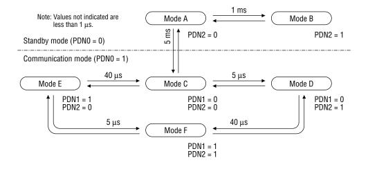
Figure 14 Transition Between Power-Down Mode and Power-ON Mode
