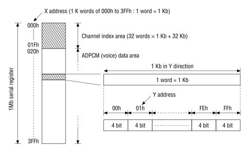
Figure 16 Address Space of 1 Mb Serial Register
