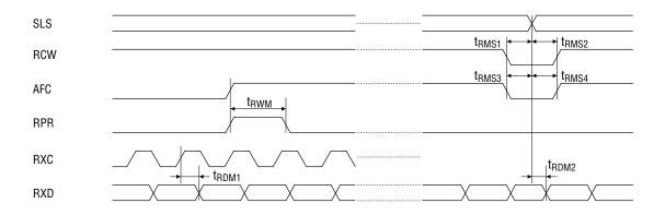
Figure 11 Receive Side (Demodulator Side) Digital I/O Timing
