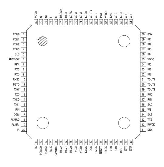
80-Pin Plastic TQFP
