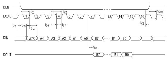
Figure 9 Serial Control Port Interface
