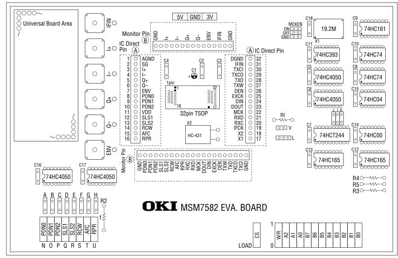
Fig. 2 MSM7582 Evaluation Board Layout
