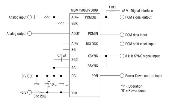
The analog output signal has an amplitude of  $\pm 1.2$  V above and below the offset voltage level of  $V_{DD}/2$ .
