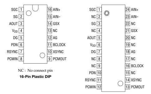
NC : No connect pin **24-Pin Plastic SOP**
