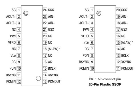
NC: No connect pin **24-Pin Plastic SOP**
