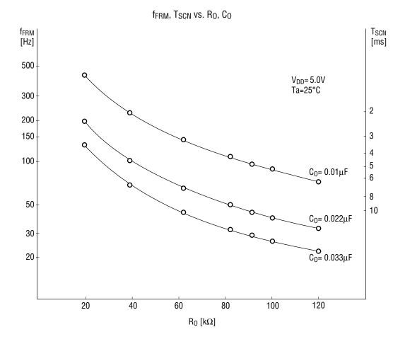
The frequency changes depending on supply voltages and temperatures. For V<sub>DD</sub>, the frequency becomes about 5% higher at 5±0.5V than at 5V. For temperature, the frequency becomes about 12% higher at Ta=-40°C and becomes about 10% lower at Ta=85°C than at Ta=25°C. (The temperature characteristic of an external resistor and capacitor is not taken into consideration here.)
