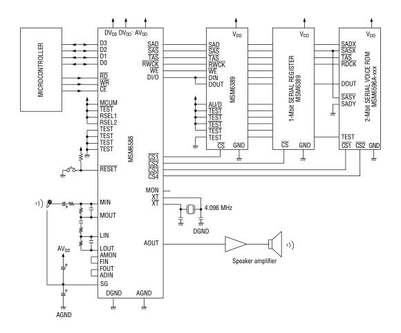
Note: When the MSM6596A is driven by the MSM6388 or MSM6588, a serial register is required. (The MSM6596A does not operate without it.) The MSM6389 is being used as the serial register in the above example.
