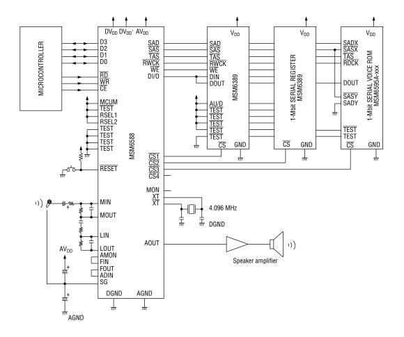
Note: When the MSM6595A is driven by the MSM6388 or MSM6588, a serial register is required. (The MSM6595A does not operate without it.) The MSM6389 is being used as the serial register in the above example.
