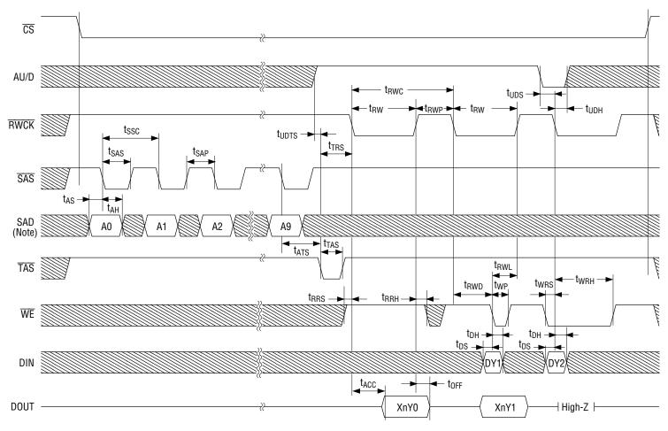
Note: Out of ten bits from A0 to A9, only the nine bits from A0 to A8 are effective. Fix A9 to "L".
