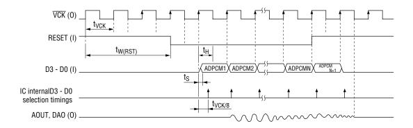
The  $\overline{\text{VCK}}$  clock rising and falling edges are reversed between the MSM5205 and the MSM6588, as indicated in DIFFERENCES BETWEEN MSM6585 AND MSM5205.
