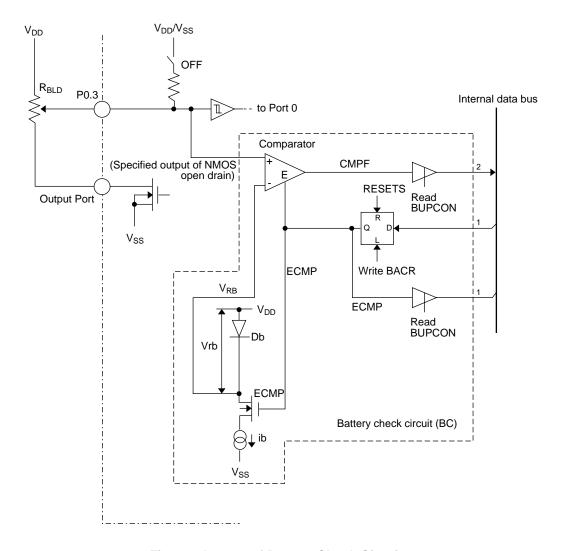
Fig. 8-1 Layout of Battery Check Circuit
