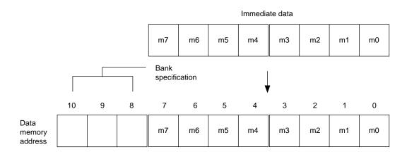
Figure 2-9 Data Memory Address of Direct Addressing
