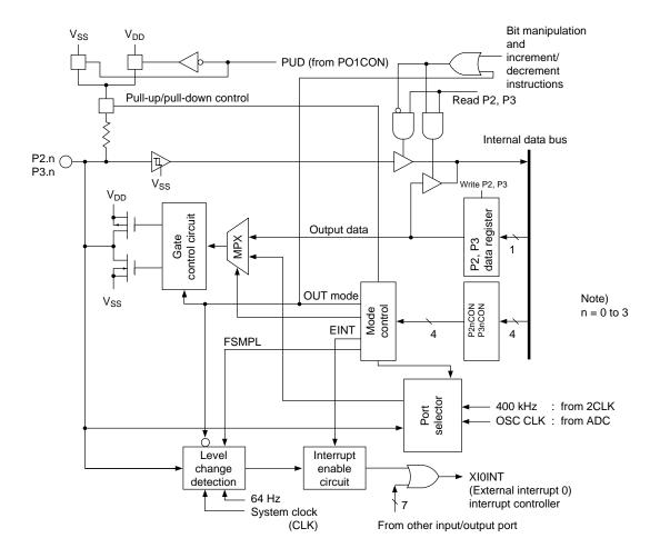
Figure 7-7 Layout of Port 2 and Port 3
