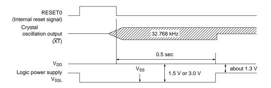
Figure 14-2 V<sub>SSL</sub> Output State in System Reset Mode
