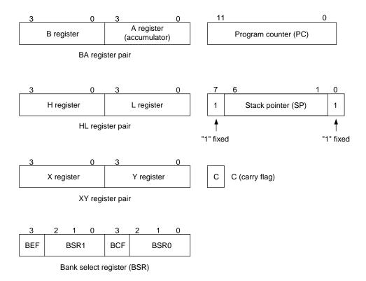
Figure 2-2 Register Layout of MSM64162A
