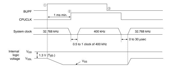
Figure 5-2 System Clock Switch Timing
