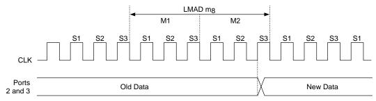
Figure 7-8 Example of Writing of Port Data Register by the "LMAD mg" Instruction
