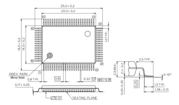
Figure C-1 80-Pin QFP
