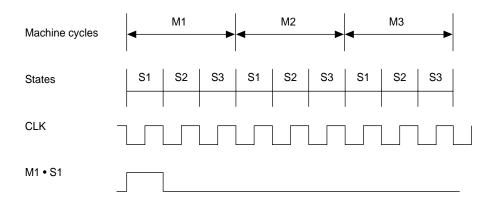
Figure 1-4 Machine Cycle Definition
