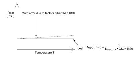
Figure 12-13 Oscillation Characteristics of Reference Resistance
