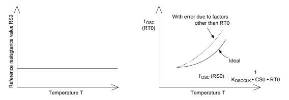
Figure 12-11 Temperature Characteristics of Reference Resistance
