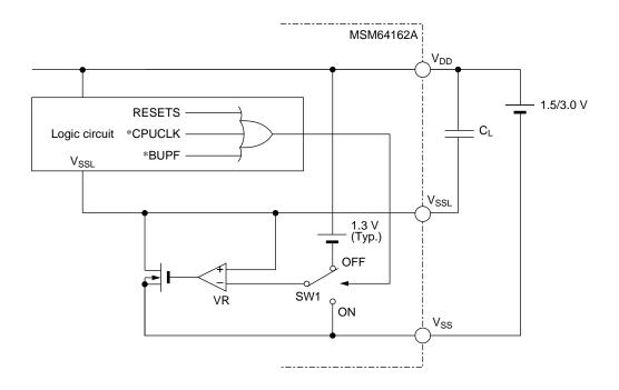
\* BUPF indicates output of the backup flag. CPUCLK indicates output of the system clock selection bit.
