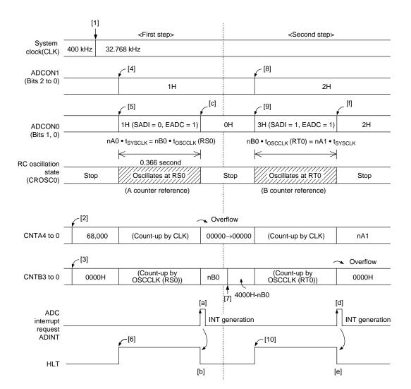
Notes: nA0 = 12,000,  $t_{SYSCLK} = 1/32768$  Hz, [1] to [10]: software processing, [a] to [f]: hardware processing
