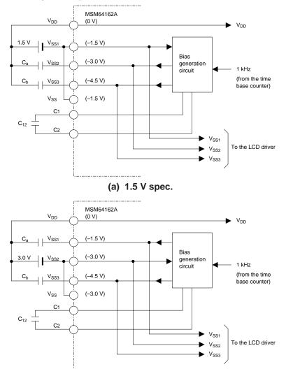
(b) 3.0 V spec. Figure 13-5 Layout of the Bias Generation Circuit
