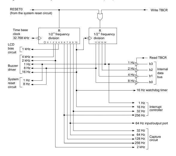
Figure 6-1 Layout of Timer Base Counter
