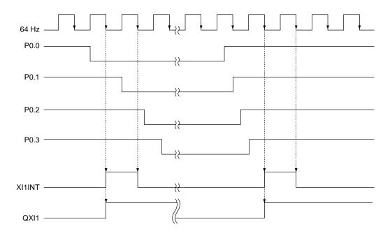
Figure 7-6 External 1 Interrupt Generation Timing (When PUD = 0)
