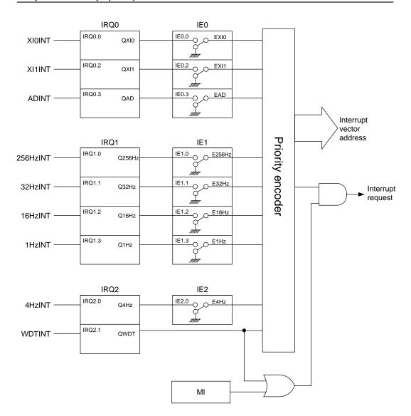
Figure 4-1 Interrupt Control Equivalent Circuit
