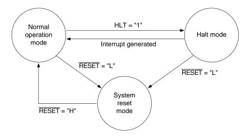
Figure 3-1 Operation Transition Diagram
