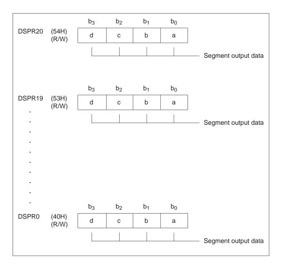
It is possible to assign an arbitrary bit of the display register to an arbitrary segment driver by the mask option. At system reset, all the display registers are reset to "0" and LCD segments are all off. Those bits set to "1" in the display register are in on state on the LCD segments while those bits reset to "0" are in off state.
