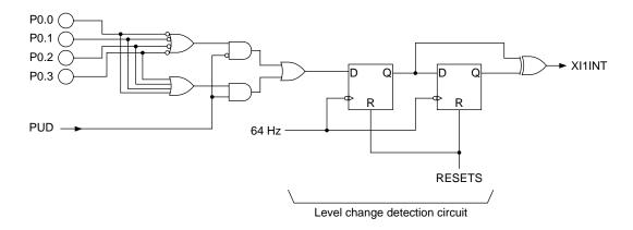
Figure 7-4 External 1 Interrupt Generation Circuit
