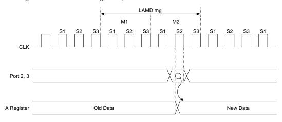
Figure 7-9 Example of Reading the Data from the Port by the "LAMD mg" Instruction
