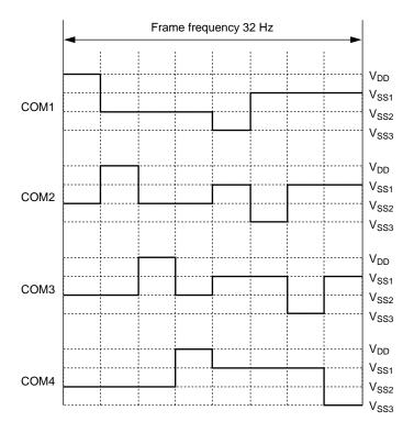
Figure 13-6 (a) 1/4 Duty Common Driving Waveforms (1/3 bias)
