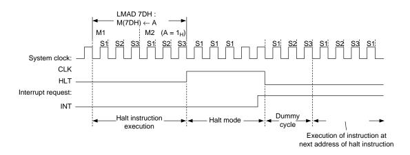
Figure 3-5 Timing of Halt Mode Set and Halt Mode Reset by Interrupt (when the MI flag = 0)
