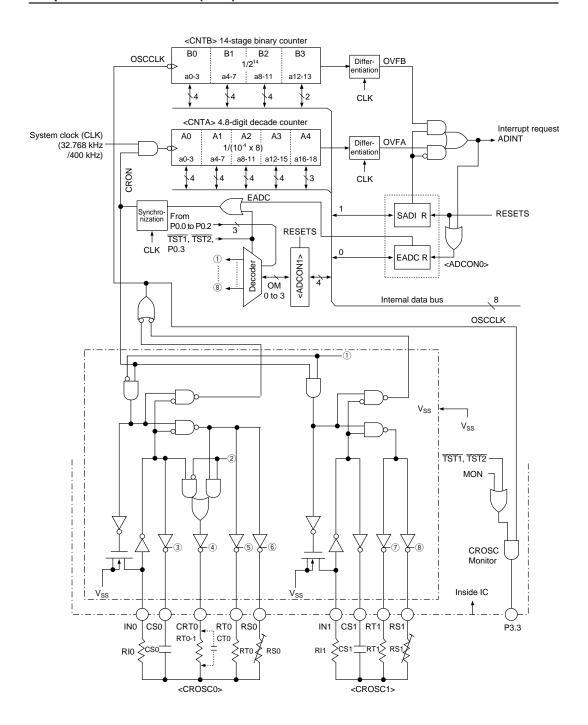
Figure 12-1 Layout of A/D Converter
