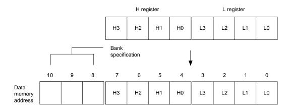
Figure 2-7 Data Memory Address of HL Indirect Addressing
