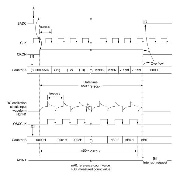
Figure 12-6 Operating Timing of Counter A Reference Mode
