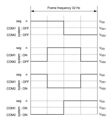
Figure 13-8 (b) 1/2 Duty Common Driving Waveforms (1/2 bias)
