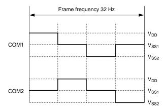
Figure 13-8 (a) 1/2 Duty Common Driving Waveforms (1/2 bias)
