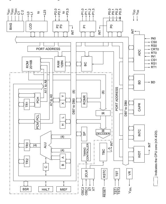
Figure 1-1 MSM64162A Block Diagram
