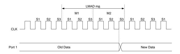
Figure 7-2 Example of Writing to Port Data Register by "LMAD mg" Instruction
