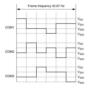
Figure 13-7 (a) 1/3 Duty Common Driving Waveforms (1/3 bias)
