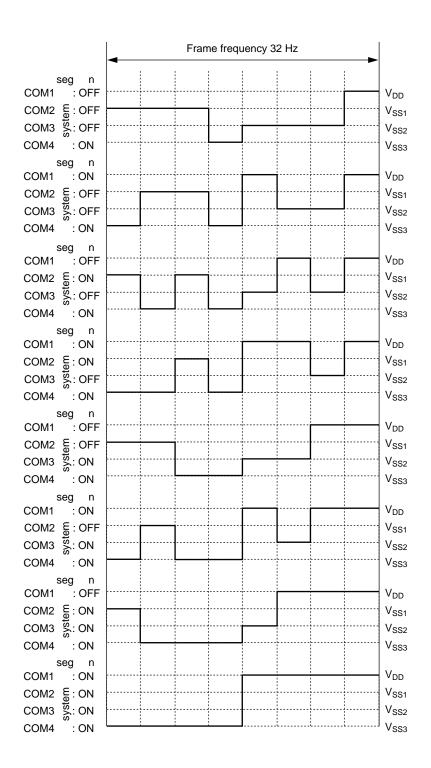
Figure 13-6 (c) 1/4 Duty Common Driving Waveforms (1/3 bias)
