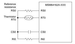
Figure 12-8 Layout of RC Oscillation Circuit of a Thermistor Using CROSC0
