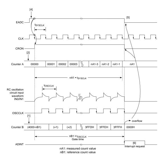
Figure 12-7 Operating Timing of Counter B Reference Mode
