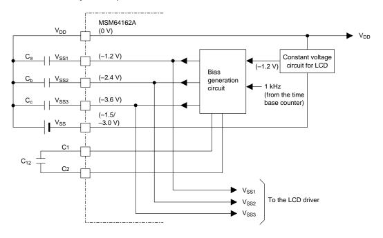
Figure 13-6 Layout of the Bias Generation Circuit (When constant voltage circuit for LCD is used) ( $C_a$ ,  $C_b$ ,  $C_c$ ,  $C_{12}$  = 0.1  $\mu$ F)
