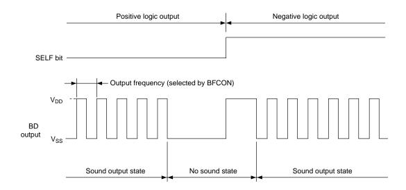
Figure 9-3 Waveform at BD Pin
