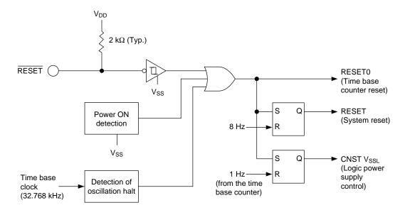
Figure 3-2 System Reset Generation Circuit
