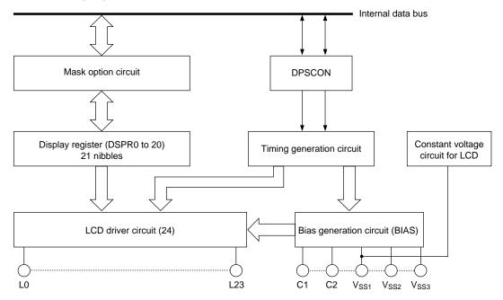
Figure 13-1 Layout of LCD Driver
