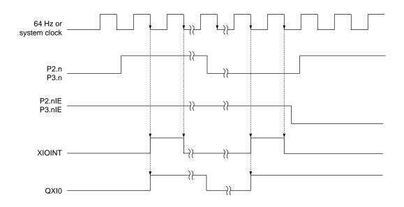
Figure 7-11 External 0 Interrupt Generation Timing
