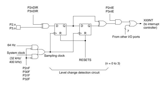
Figure 7-10 External 0 Interrupt Generation Circuit (one bit)
