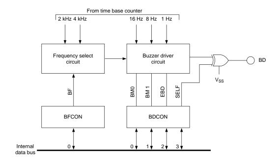
Figure 9-1 Layout of Buzzer Driver
