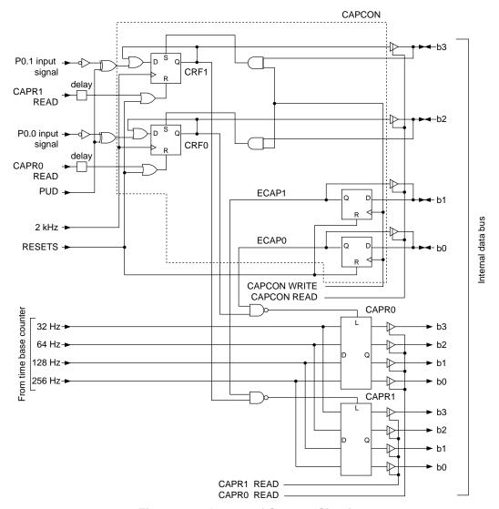
Figure 10-1 Layout of Capture Circuit
