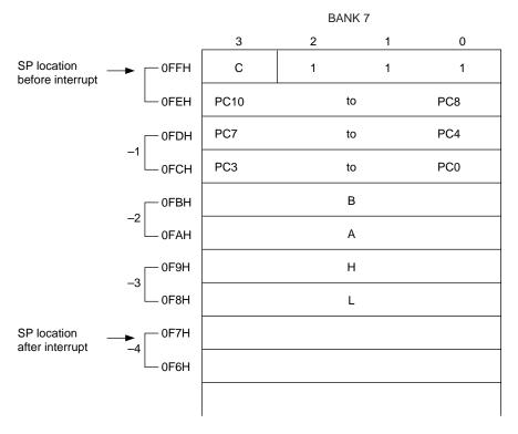
Figure 4-2 Contents of Stack after Interrupt Generation
