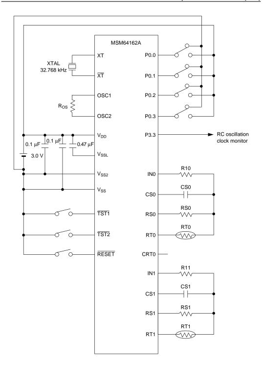
Figure 15-2 Connection Example of Test Mode (3.0 V operation mode)
