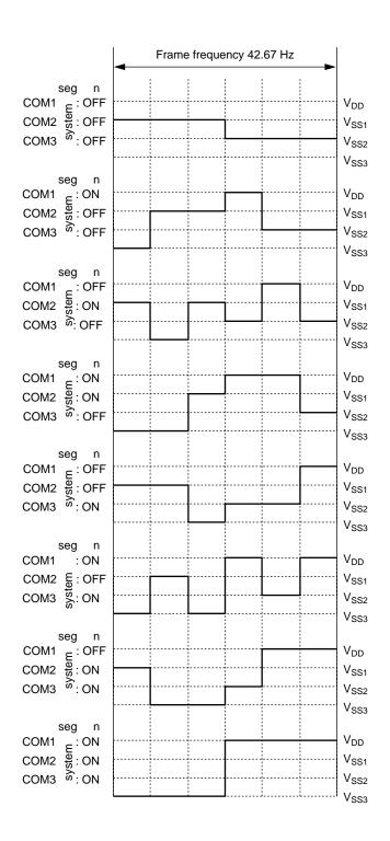
Figure 13-7 (b) 1/3 Duty Common Driving Waveforms (1/3 bias)
