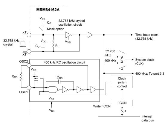
Figure 5-1 Layout of Clock Generation Circuit
