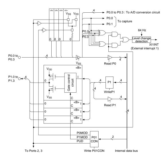
Figure 7-1 Layout of Port 0 and Port 1
