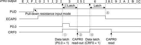
Figure 10-2 Data Latch Timing of Capture Data Register 0 (CAPR0)
