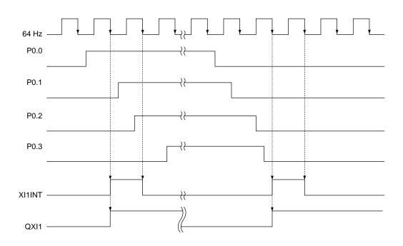
Figure 7-5 External 1 Interrupt Generation Timing (When PUD = 1)
