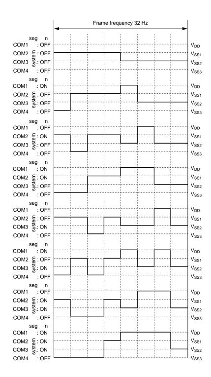
Figure 13-6 (b) 1/4 Duty Common Driving Waveforms (1/3 bias)
