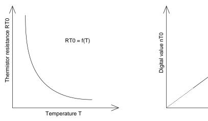
Figure 12-9 Temperature Characteristics of Thermistor
