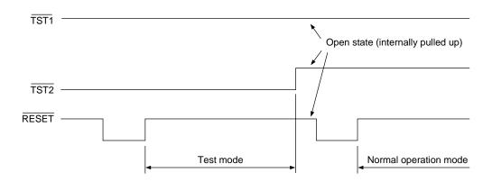
Figure 15-1 Relationship among the TST1, TST2 pins and the RESET pin
