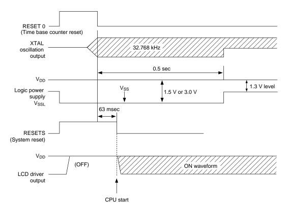
Figure 3-3 Each Signal at System Reset Generation
