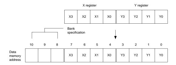
Figure 2-8 Data Memory Address of XY Indirect Addressing
