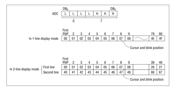
(Note) The cursor and blink are displayed even when the CG RAM address is set in the ADC. For this reason, it is necessary to inhibit the cursor and blink display while the CG RAM address is set in the ADC.
