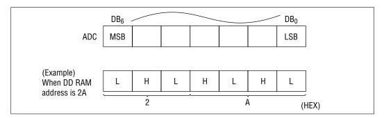
(1) Correspondence between address and display position in the 1-line display mode
