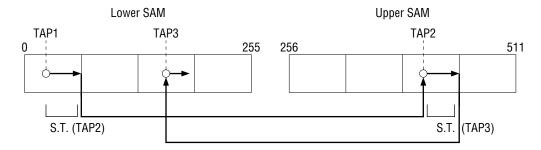
Figure 2. Example of Boundary Split Register
