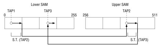
Figure 2. Example of Boundary Split Register
