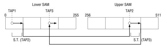
Figure 2. Example of Boundary Split Register
