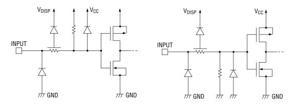
• Schematic Diagrams of Logic Portion Output • Schematic Diagrams of Driver Output Circuit Circuit
