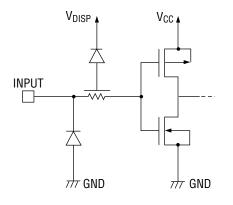
• Schematic Diagrams of Logic Portion Input Circuit (Pull-up) • Schematic Diagrams of Logic Portion Input Circuit (Pull-down)
