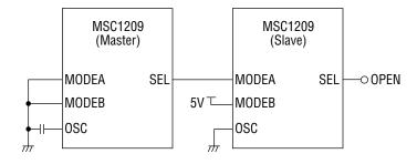
The IC where the MODEA and MODEB pins are set to "L" operates as the master, and the one where the MODEB pin is set to "H" as the slave.
