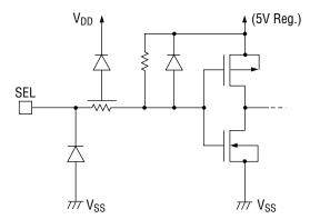
• Schematic Diagram of Logic Portion Output • Schematic Diagram of Driver Output Circuit Circuit
