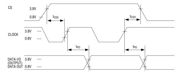
Figure 2 Data Output Timing
