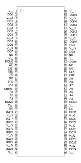
86-Pin Plastic TSOP (II) (Type K)
