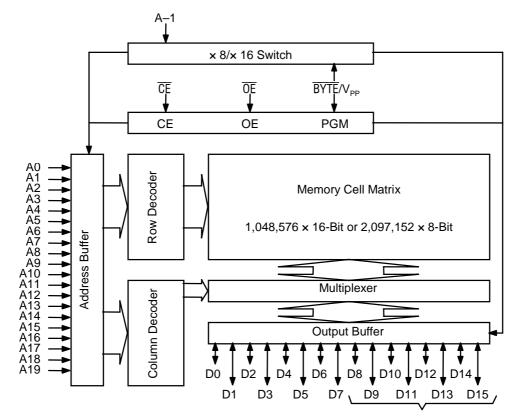
In 8-bit output mode, these pins are placed in a high-Z state and pin D15 functions as the A-1 address pin.
