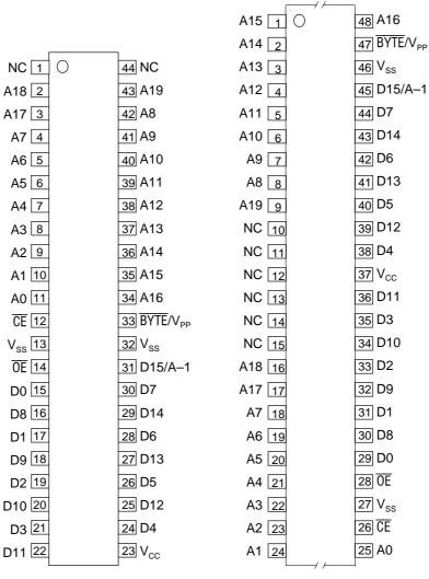
44-pin SOP, TSOP(II) 48-pin TSOP(I)
