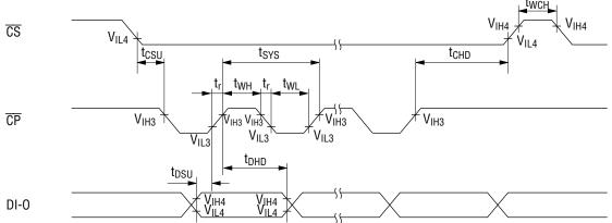
Clock synchronous serial interface input/output timing
