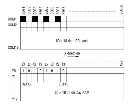
Figure 2 Correspondence Between Display Screen and Memory
