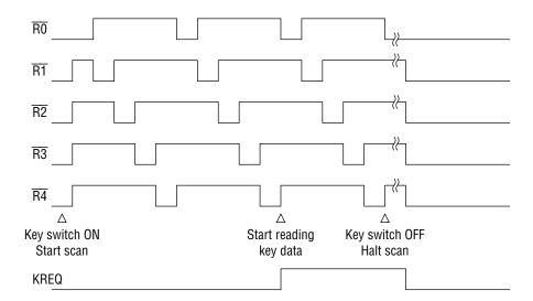
Note 1: Pressing three or more key switches simultaneously may result in incorrect recognition (a switch that was not pressed may be recognized as a switch that was pressed). Therefore, if it is necessary to recognize three or more pressed switches, connect a diode in series with each switch. If three or more pressed switches are not to be recognized, data should be ignored if there are three or more "1s" in the key data that is read by software.
