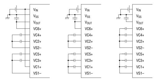
5-times voltage multiplier circuit 6-times voltage multiplier circuit 7-times voltage multiplier circuit
