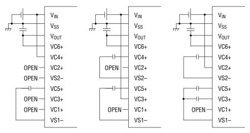
2-times voltage multiplier circuit 3-times voltage multiplier circuit 4-times voltage multiplier circuit
