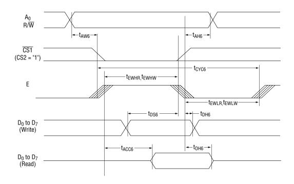
$[V_{DD} = 4.5 \text{ V to } 5.5 \text{ V}, \text{ Ta} = -40 \text{ to } +85^{\circ}\text{C}]$
