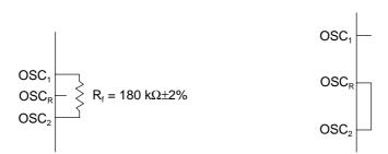
The wire between  $OSC_1$  and  $R_f$  and the wire between  $OSC_2$  and  $R_f$  should be as short as possible. Keep  $OSC_R$  open.
