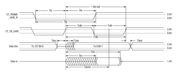
Figure 15. H.100/H.110 Detailed Data Bus Timing
