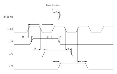
Figure 11. Local Clock and Frame Synchronization Timing
