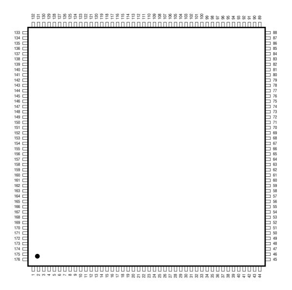
Figure 1. ML53612 176-Pin LQFP Pin Configuration
