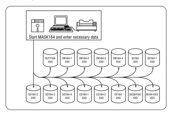
Figure 1-2 Mask Option Data File Generating Process
