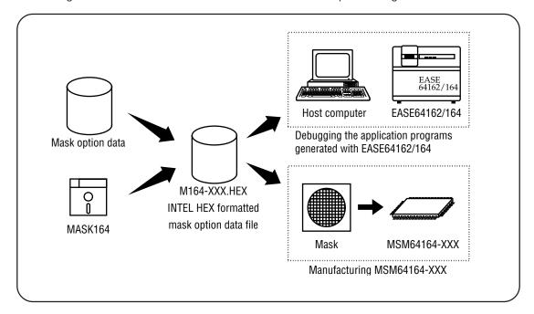
Figure 1-3 Use of Mask Option Data Files
