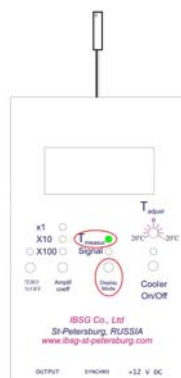
Fig.6. The button of display mode selection and the LED indicator of the PD temperature indication mode.
