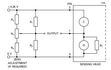
Fig. 1 Recommended circuit diagram
