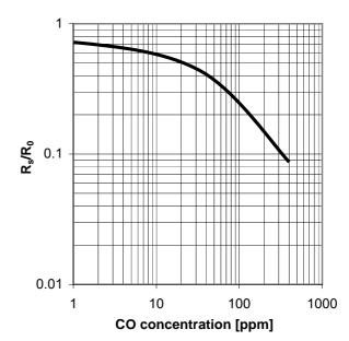
Figure 2:  $R_s/R_0$  as a function of CO concentration at 40% RH and 25 °C, measured on an engineering test bench
