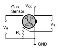
Figure 3: MiCS-5525 with measurement circuit (top view)
