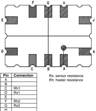
Figure 1: MiCS-5524 configuration (bottom view)
