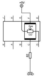
Figure 2: MiCS-5524 with recommended supply circuit (top view)
