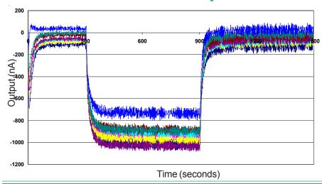
When designed with a 22 ohm load resistor, the NO2-B1 shows excellent resolution, even at the ppb level: ideal for outdoor air environmental testing.
