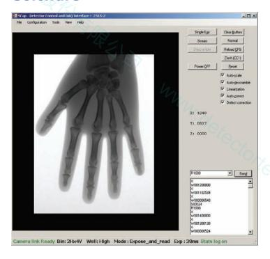
Dexela provides software drivers and companion software with its detectors. The software includes a basic application for image acquisition and viewing on a workstation or laptop running Microsoft Windows XP or Vista (x32 or x64). The development kit includes the Dexela SCAP software application that performs detector calibration, sensor set-up, image acquisition and image corrections. SCAP includes file translators for smv, raw and tif formats.
