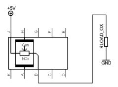
MiCS-2714 with recommended supply circuit (top view)
