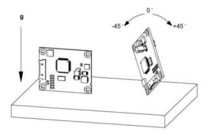
Figure 5-2: Accelerometer Calibration Starting Orientations
