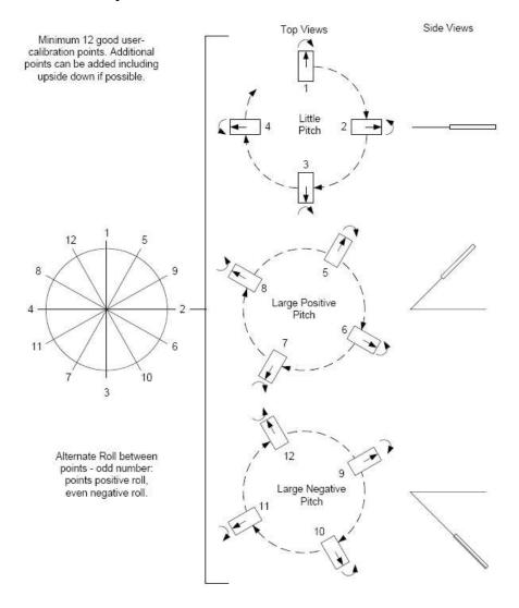
Figure 5-1: 12 Point Full Range Calibration
