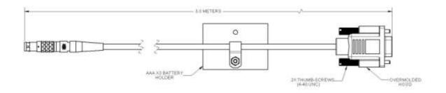
Figure 3-6: Trax RS232 Cable Drawing
