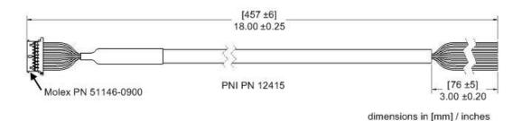
Figure 3-3: PNI Pigtailed Molex Cable Drawing
