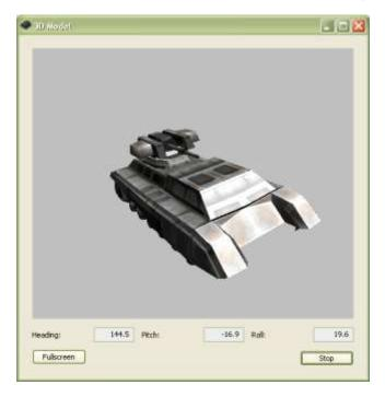
Clicking the <Start> button begins continuous updating of the orientation of the rendered model, and of the heading, pitch, and roll output fields. The <Start> button on the Test Tab screen and on the 3D Model screen are linked such that selecting either of them will stop or start both screens.
