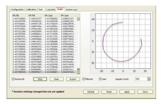
The "Filt" data and plot (blue) provides magnetic field strength measurements after the FIR filter taps are applied, but prior to applying the user calibration coefficients. The "User" data and plot (red) provides data after applying the user calibration coefficients. In AHRS Mode the data and plots are identical, while in Compass Mode there is an offset which represents
