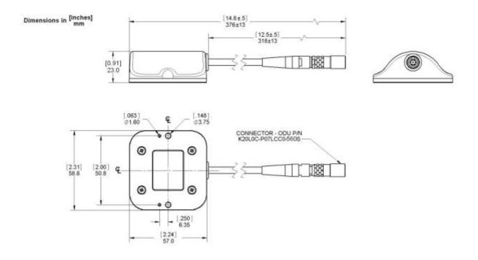
Figure 3-4: Trax Enclosed Mechanical Drawing
