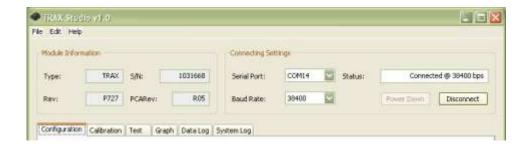
To connect, set the "Serial" field to the appropriate COM port. To determine this, in Windows right click on "My Computer", select "Manage", then select "Device Manager". Expand "Ports" and note the port for "USB Serial Port". This should be the assigned COM port for the Trax.
