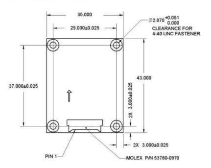
Figure 3-2: Trax PCA Mechanical Drawing
