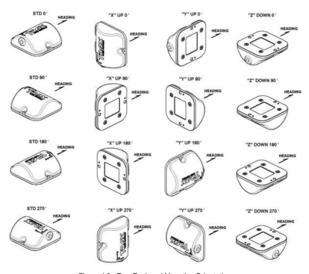
Figure 4-2: Trax Enclosed Mounting Orientations
