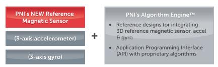
The SpacePoint 9-axis sensor system consists of 3 separate sensors that are driven by PNI's Algorithm Engine for Exact Gesture Responsiveness.
