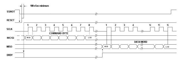
Figure 5-1: SPI Port Full Timing Sequence
