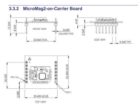
Figure 3-7: MicroMag2-on-Carrier Mechanical Drawing
