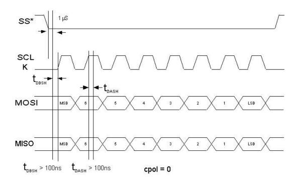
Figure 5-2: SPI Port Timing Parameters
