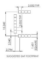
Figure 3-5: MicroMag2 Suggested SMT Footprint
