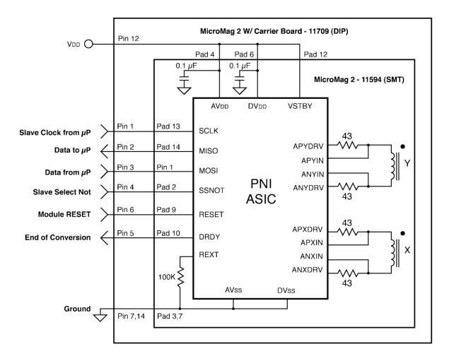
Figure 4-1: MicroMag2-on-Carrier Reference Block Diagram
