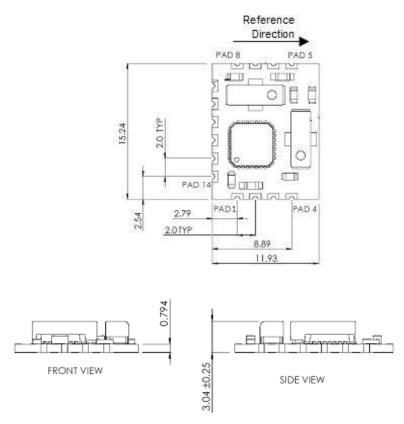
Figure 3-4: MicroMag2 Mechanical Drawing
