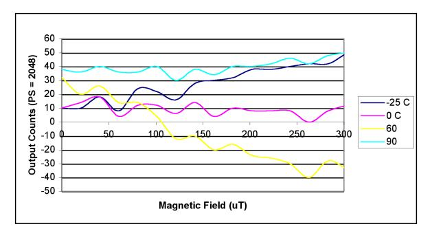
Figure 3-3: Linearity vs. Temperature, Normalized to Room Temperature
