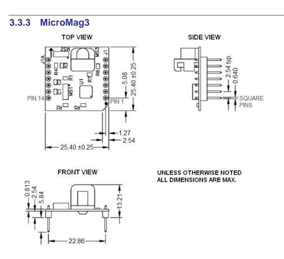
Figure 3-9: MicroMag3 Mechanical Drawing
