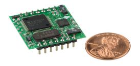
perfect solution for adding compass heading functionality to virtually any application — from hobbyist projects and consumer electronics prototypes to high-performance solid-state navigation and magnetic field sensing equipment.
