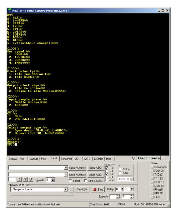
6. Power on the RM3000 Evaluation Board by typing "W" <CR>. You can use the SPI> prompt or the boxes on the Send tab and Send ASCII button.
