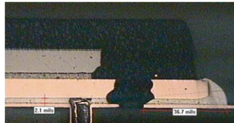
81% paste coverage, encroached via, 2.1 mil standoff
