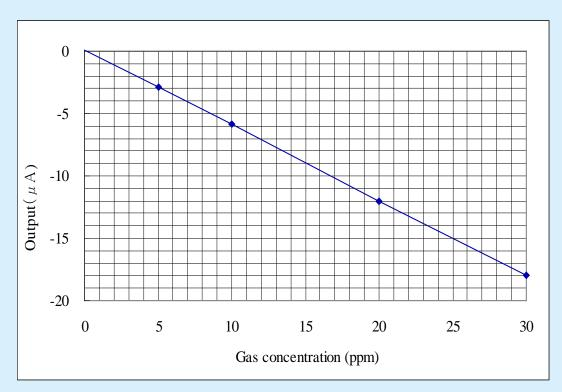
Fig.2: Gas Sensitivity of NE4-NO2
