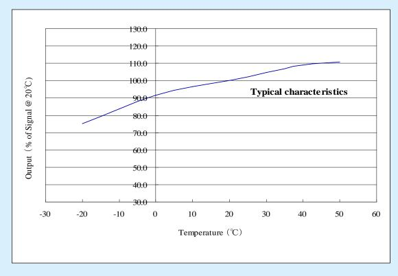
Fig. 3 : Typical temperature coefficient of NE4-NO2 (100 at 20 degree C)
