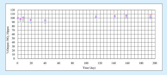
Fig.8: Durability in low temperature (-20 degree C)
