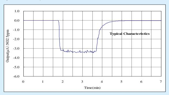
Fig.4 : Response and recovery characteristics of NE4-NO2 (at 20 degree C)
