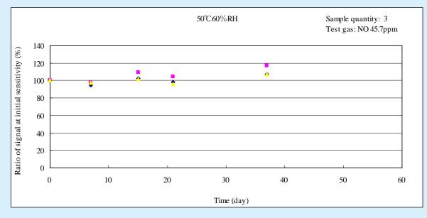
Fig.9: Durability in high temperature (50°C) and normal humidity (60%RH)
