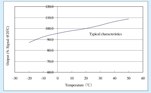
Fig. 4 : Typical temperature coefficient of NE4-NO (100 at 20 °C)
