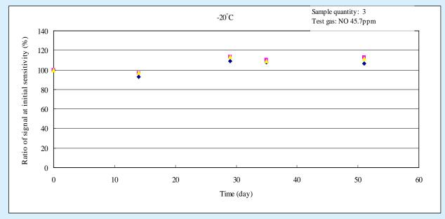
Fig.10: Durability in low temperature (-20°C)
