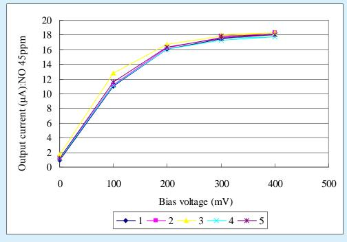
Fig.6: Bias supply voltage dependence
