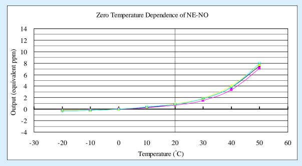
Fig. 3 : Zero temperature dependence of NE4-NO
