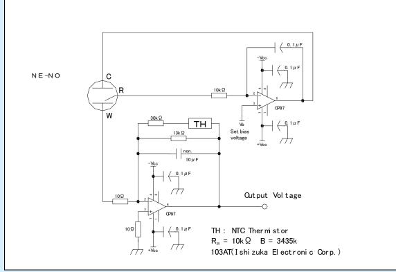
Fig. 11: Measuring circuit diagram for evaluation
