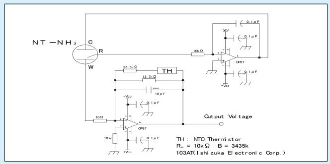
Fig. 10 : Measuring circuit diagram for evaluation
