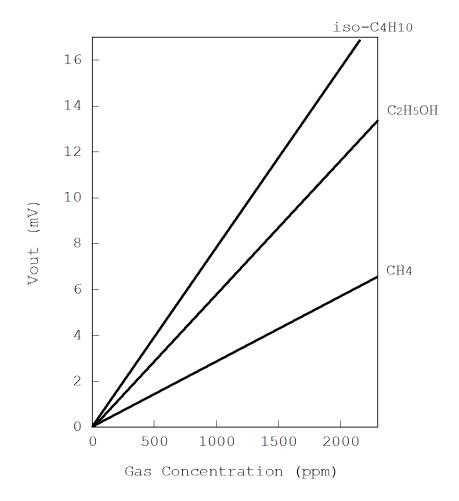
For other flammable gases, Nemoto can advise on the anticipated sensitivity of the sensor alone, but since the relative sensitivities to various gases is also dependent on the mounting arrangement within an instrument, it is always recommended that the instrument maker determines the response of the sensor to the target gas by experiment using the final product design wherever possible.
