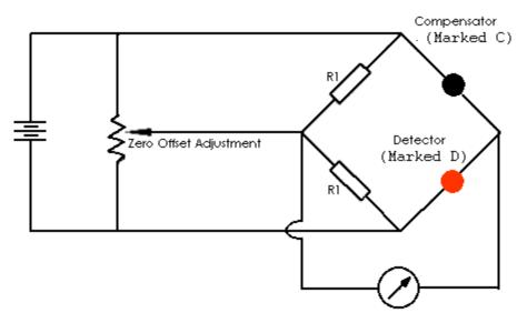
Pellistor Drive/Measurement Circuit: A simple Wheatstone Bridge to compare the resistance of two hot elements
