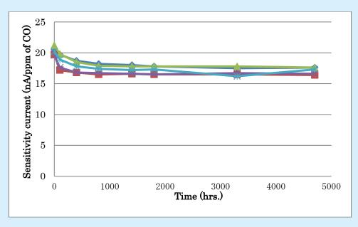
The sensors in this test were then stored in normal room condition to allow the electrolyte to re-establish a normal equilibrium. After a further 4 weeks in these conditions, the sensors were retested to confirm that the sensors had suffered no significant effect on their performance. The sensitivity signal of the sensors before and after the test is illustrated in the table below:
