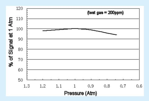
The Figure below represents the effect of altitude on the sensitivity of the NAP-508:
