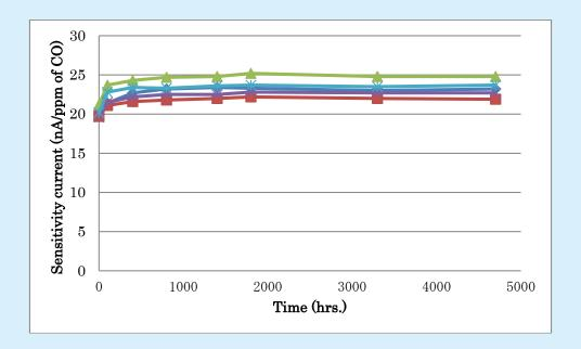
The sensors in this test were then stored in normal room condition to allow the electrolyte to re-establish a normal equilibrium. After a further 4 weeks in these conditions, the sensors were retested to confirm that the sensors had suffered no significant effect on their performance. The sensitivity signal of the sensors before and after the test is shown in the table below:
