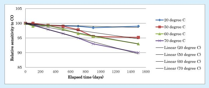
Extrapolating from the data above, it is possible to estimate the lifetime at 25 deg C by plotting the activation energy of the sensor against time. Using this method, the lifetime of the sensor is estimated at 63 years as illustrated below:
